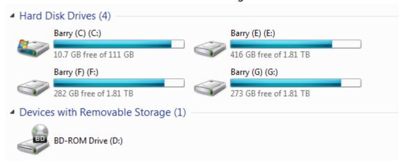
Drive C is a Solid State Drive (SSD) for speed of access, 120GB capacity, stores programmes only
